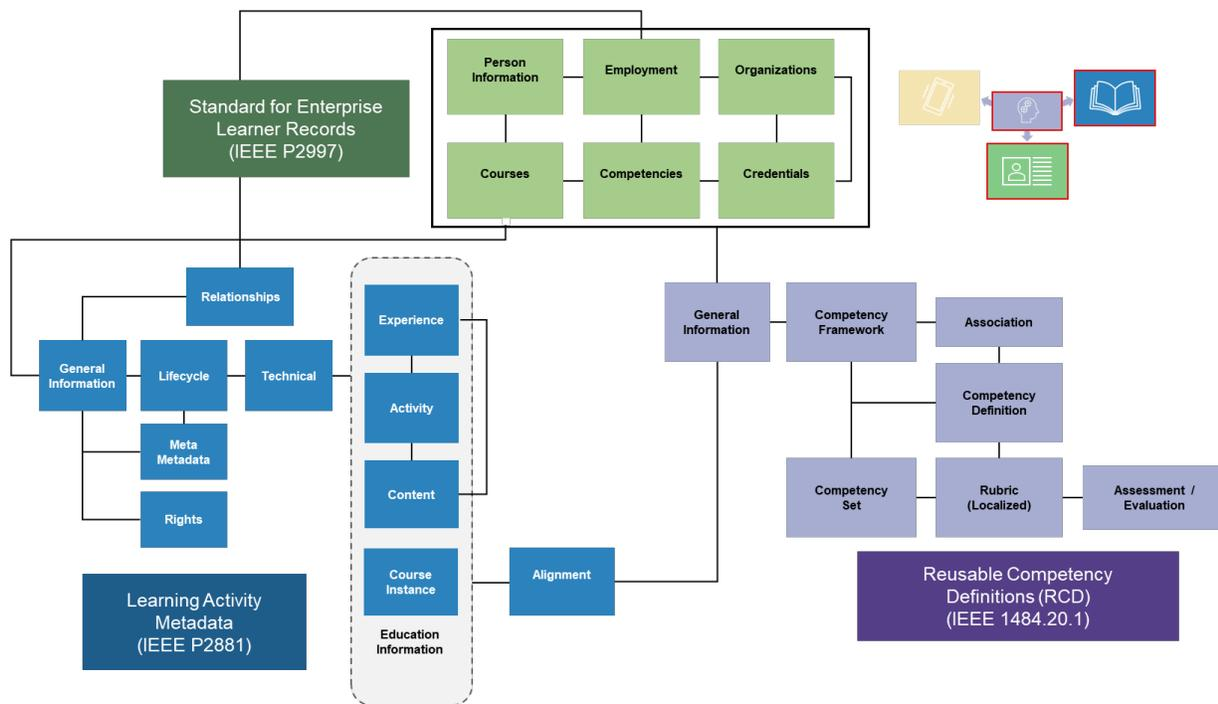
**Figure 1. Total Learning Architecture's Logical Data Model (Partial View).** This image shows the major subcomponents of three of the four TLA data pillars. It omits xAPI, the data standard for collecting runtime performance, which is discussed later in the paper.
