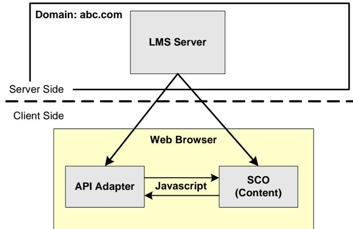
Figure 3.1a – One LMS/Content server with no virtual IP addresses
