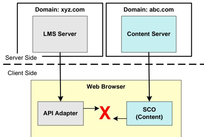
Figure 3.2a – Separate LMS server and Content Server
